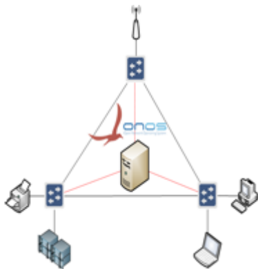
ON.Lab local office network Reactive forwarding
